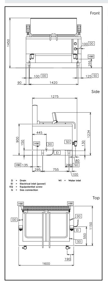
**Electric** Supply voltage: 291161 (CR42G) 230 V/1N ph/50 Hz Gas Gas Power: 60 kW Gas Type Option: LPG; Natural Gas Gas Inlet: 1"1/4 **Key Information:** Number of wells: 2 Usable well dimensions (width): 625 mm Usable well dimensions (height): 410 mm Usable well dimensions (depth): 640 mm 190 It MIN; 190 It MAX Well capacity: External dimensions, Width: 1600 mm External dimensions, Depth: 1280 mm External dimensions, Height: 850 mm Net weight: 386 kg
